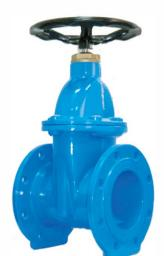
Gate Valves, Resilient seated, full bore, Inside screw bolted bonnet, Fully removable part, Free maintenance, 100% water tight Non Rising Stem
