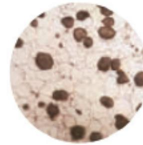
Ductile cast iron metallographic
