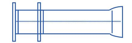
Flange Socket Pipe with Puddle Flange
