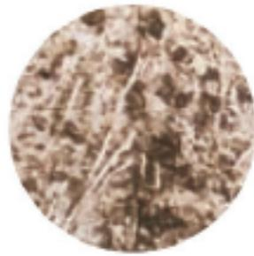
Ductile cast iron metallographic
